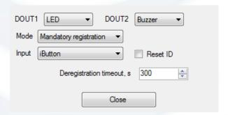
Deregistration means period of time, when you can start engine again without need to register again. For example, deregistration is set to 300 seconds (5 minutes). If engine is turned off, it can be started again within 5 minutes without registration.
