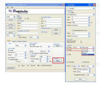
You can select up to 3 source inputs. Port A RS232 interface, Port B RS232 interface and iButton connected to 1-Wire interface.
