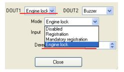
Select engine lock, then choose *input* source (iButton, RFID port A, RFID port B). Now if driver register authorized card or ibutton, he is allowed to turn on ignition and start engine.
