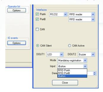
Now, if you selected iButton as mandatory registration source, driver will have to register in order to drive. If driver is not identified in 5 seconds after starting engine, peripherals connected to DOUTs start to indicate. In example shown, LED will glow red and buzzer begins making sound alert until registration is made or engine is off. Other registration sources (RFID port A and RFID port B) will register card ID without any authentication and send record to tracking platform.
